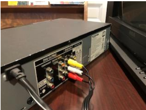
Connecting the RCA cables to their respective OUTPUTS on the VCR.
