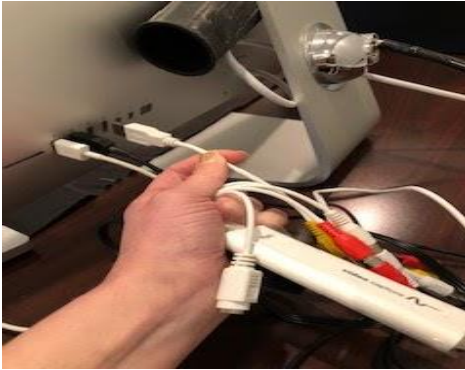
Connecting the Elgato Video Capture USB cable to the computer.
